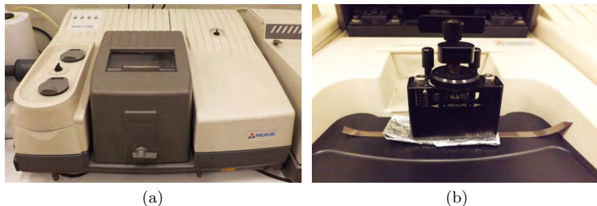
Fig. 7.5: (a) Equipment used for the FTIR analysis; (b) detail of the tape sample in position during the analysis.
