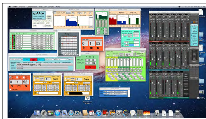
Fig. 12.13: Screenshot of the patch developed in Max/MSP for the re-installation of Andriano Guarnieri's "Medea" in 2012. The spatialization is controlled with the module SpAAce, developed by Mo. Alvisè Vidolin.
