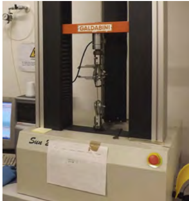
Fig. 7.10: The instrument used for the tensile test: a dynamometer Galdabini SUN2500 with a load cell of 25,000N. Author of the picture: Federica Bressan. Location: Department of Industrial Engineering (chemical sector), University of Padova.
