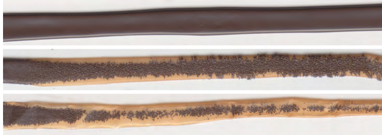
Fig. 9.6: Different degrees of deformation of a magnetic tape during a tensile test.
