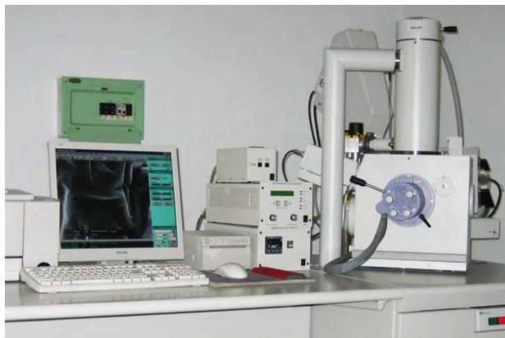
Fig. 7.7: The instrument used for the SEM and ESEM analyses at the Centro Universitario Grandi Apparecchiature Scientifiche (CUGAS) of the University of Padova. Source of the picture: Department of Industrial Engineering (chemical sector), University of Padova. Location: CUGAS.
