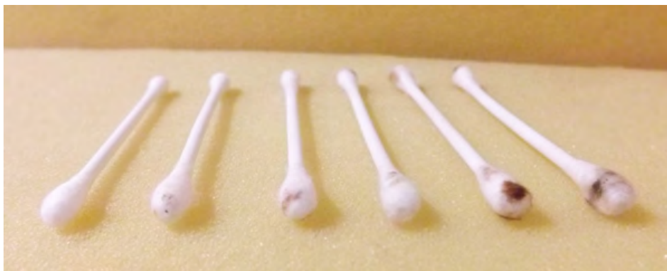
Fig. 7.4: Cotton buds used to remove the sticky residue caused by SBS-SSS from the audio heads of a ree-to-reel recorder. From left to right, the quantity of residue removed increases, making the cotton buds more dirty. Gaining experience by evaluating the quantity of residue helps to plan better treatments for the tapes affected by SBS-SSS. Author of the picture: Federica Bressan. Location: Centro di Sonologia Computazionale (CSC), University of Padova.
